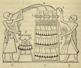
458. Siphons used about the year 1430 n.c. Thebes. 1 Pours a liquid into vases from the cup b; and 2 draws it off by the siphons a.
