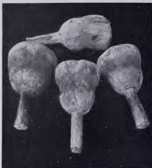
FIG. 41.—Collection of Ancient Wooden Mallets used by the Egyptian stone-masons.
